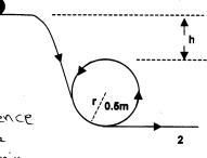
$\Rightarrow h = \frac{V_{min}^2}{29} = \frac{r}{2} = \frac{0.5}{2} = 0.25 \text{ m}$ (b) At position 1  $E_i = mgh$
